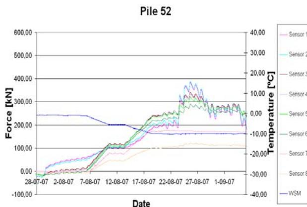
**Figure 5: Relation temperature and pile forces**
