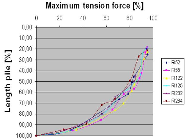
**Figure 8: Load distribution in the piles in percentages of the maximum load**
