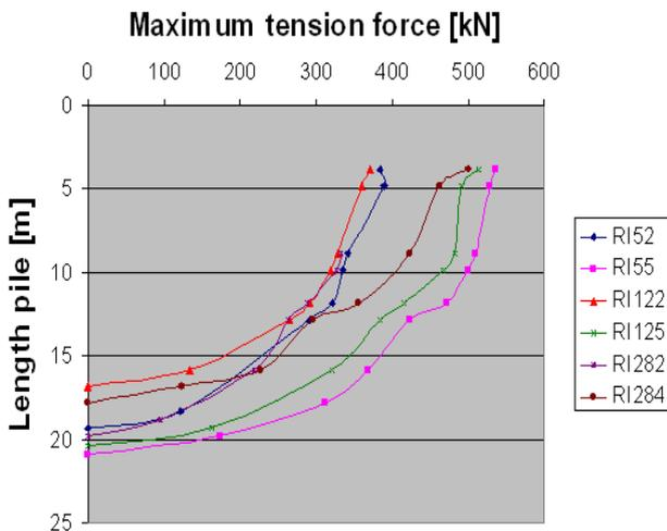
**Figure 7: Load distribution in the piles**
