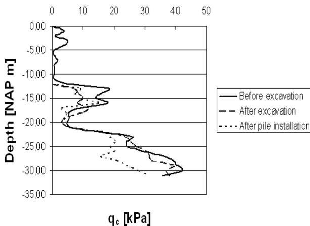
**Figure 10: Cone Penetration Tests**
