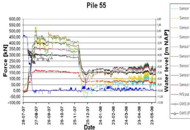
**Figure 4: Forces along the shaft**
