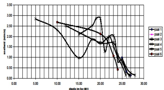
Figure 3: Penetration rate testing piles
