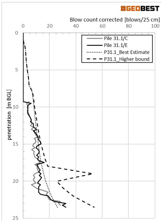
Fig. 12. Blow count corrected vs depth, pile 31.1 (Jetty C)
