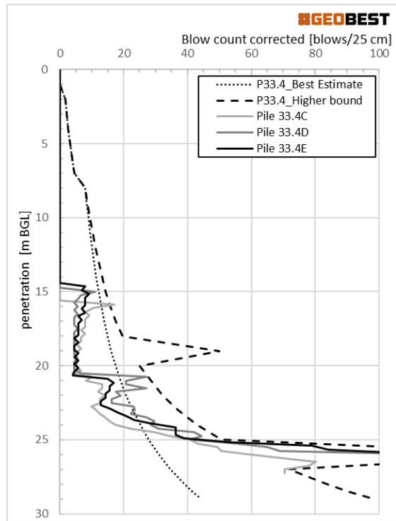
Fig. 13. Blow count corrected vs depth, pile 33.4 (Jetty C)
