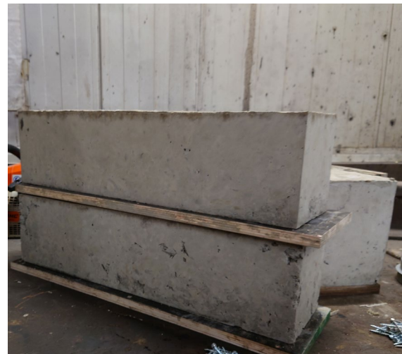
Figure 2 – Sample of stabilised foam glass.
