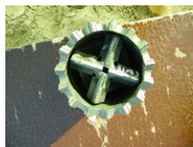
A Double drill casing with internal flush
